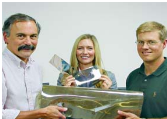
TWISTED NanoSonic's Claus (from left), Lalli, and Jeff Mecham demonstrate the flexibility of Metal Rubber, which also is reflective and conducts electricity.
