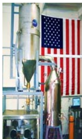
POWERED UP QuantumSphere makes metallic nanopowders for the military and, potentially, for energy storage. The reactor is on the right; the collector, on the left.
