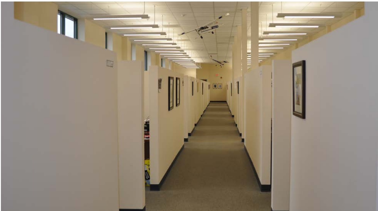
Daylighting is facilitated with large windows on the south wall and supplemented by sensed lighting that automatically turns off and on based on motion detection.
