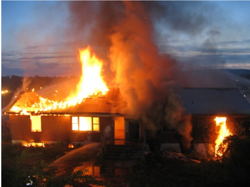
The right side of a derelict building was treated with HybridShield.
